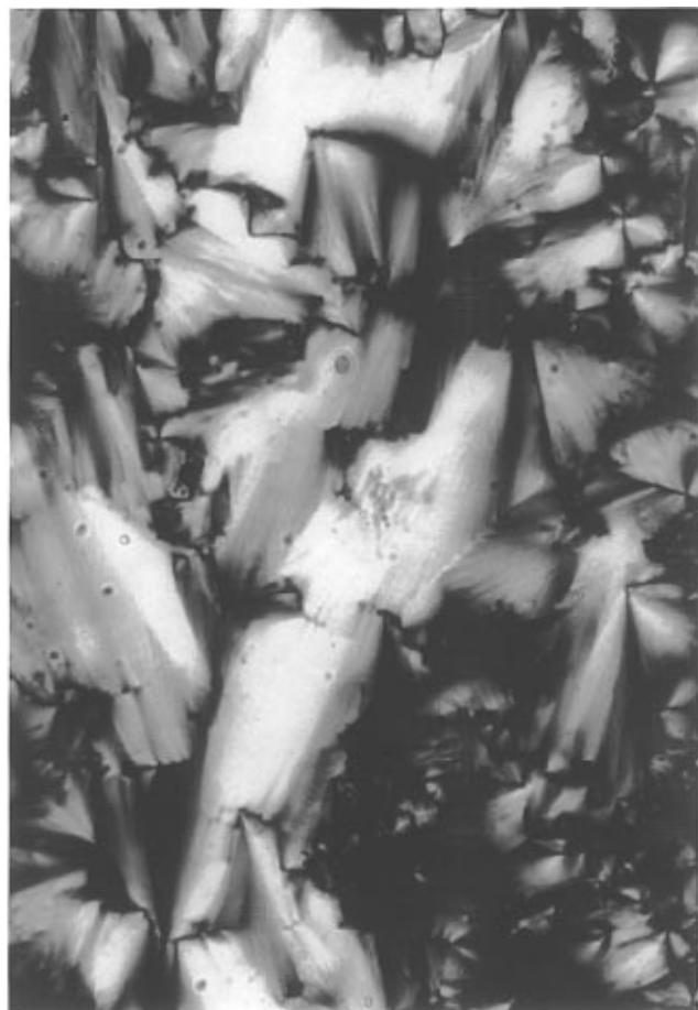
Figure 4. Smectic fan-shaped texture of I-6,6-F8H4,Me/Br at 493 K as observed by polarizing optical microscopy.
